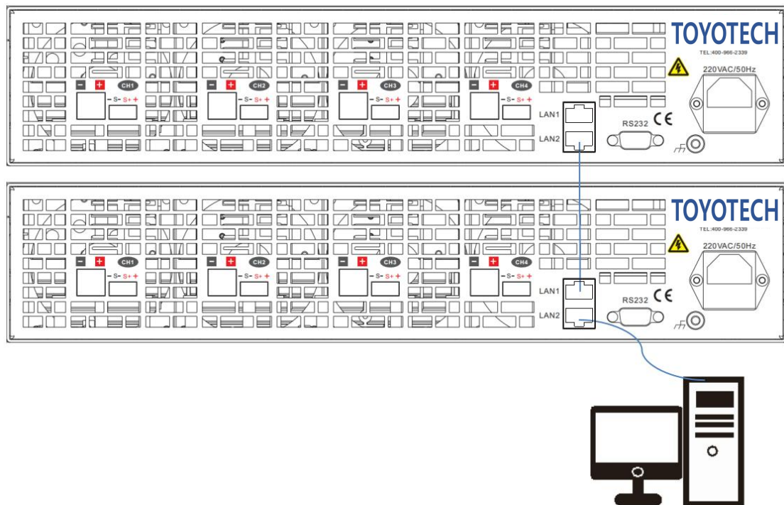
Figure 2 Multiple Devices Connection Diagram
